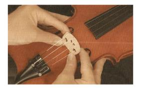
The bridge should be located between two sound holes, and the trailing edge of its two feet is cut on the ligature of the inner notch of the two sound holes As shown in the figure:
